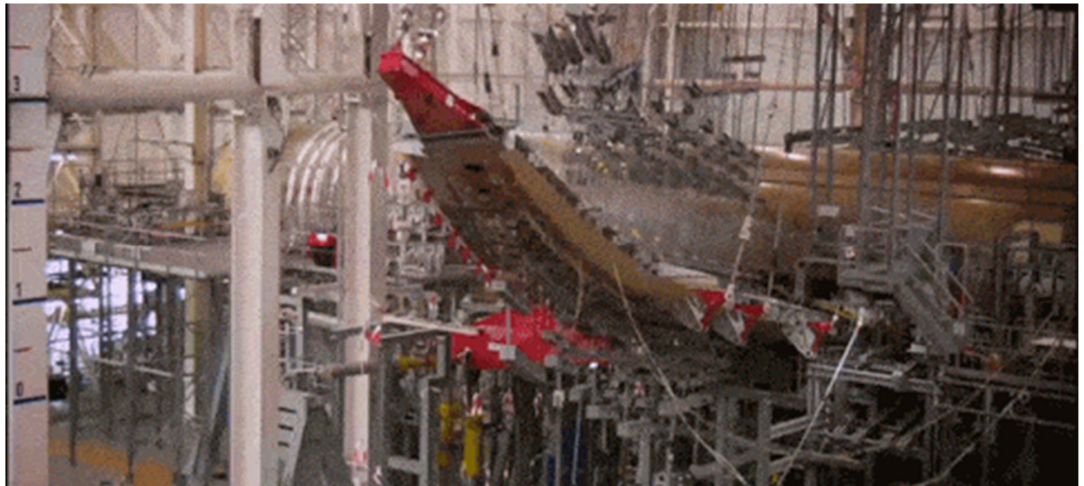
A350 Wing-Up Bending Test - Quelle: Popular Mechanics
